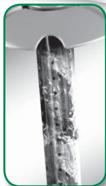
Termites are present inside the stake
